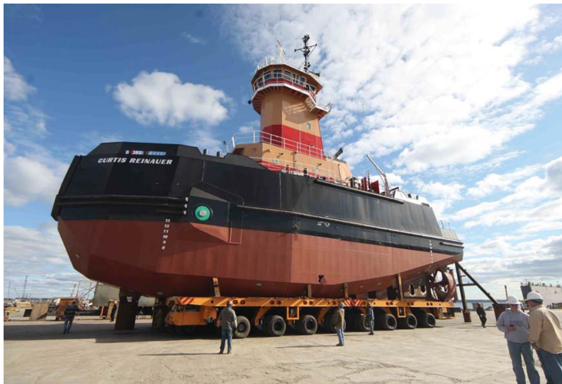
Curtis Reinauer tug built by Senesco Marine. (110' L x 33' B x 18' D)
