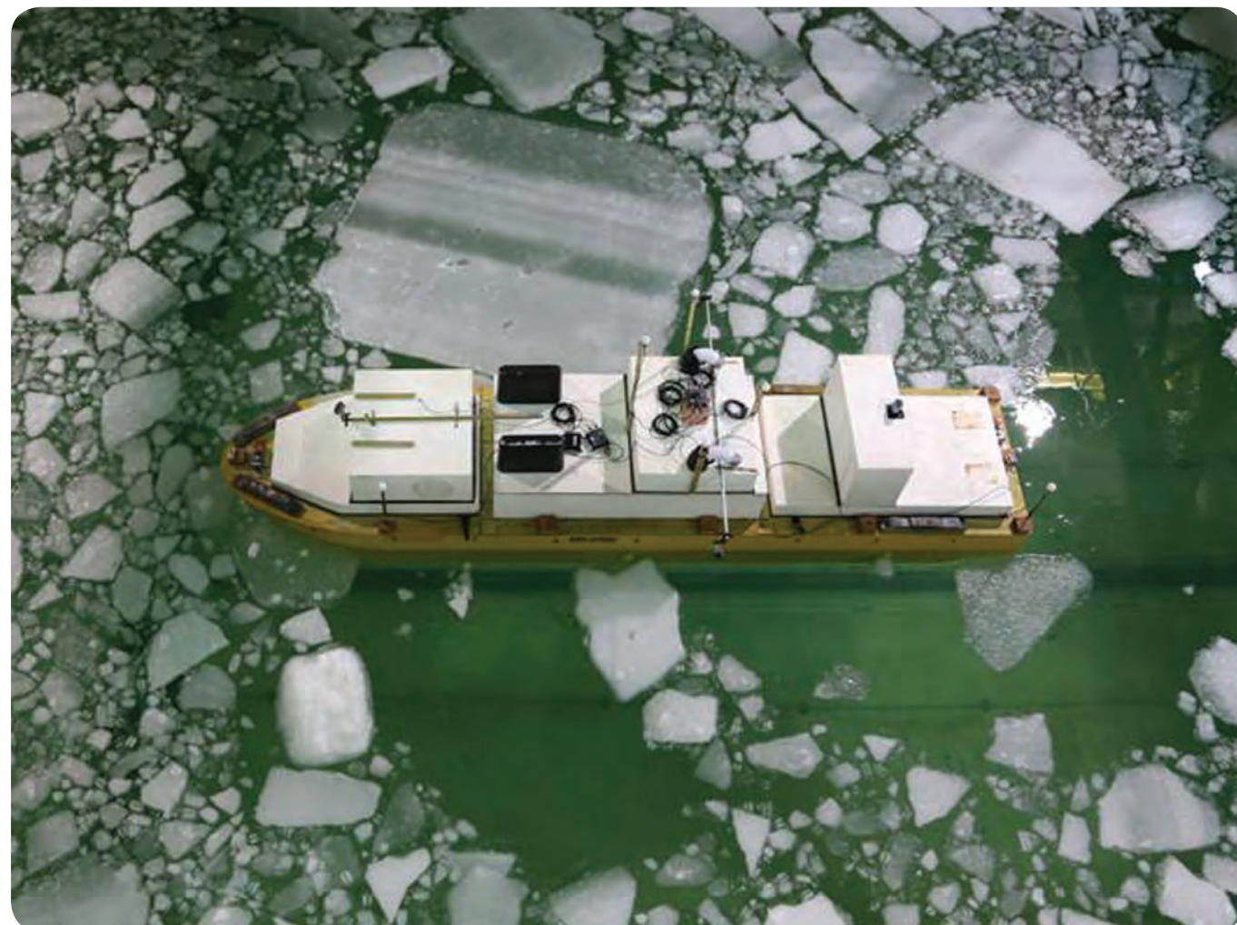
Model moving through complex ice field. A model scale 100-m floe is next to the vessel.
