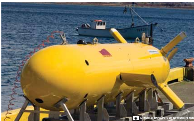
Memorial University of Newfoundland's Explorer AUV is designed with a 3,000 metre depth capability and can carry 200 kg of scientific equipment.
