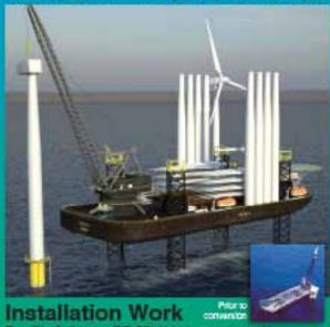
Zee Rig 3 (former DB-23) is being upgraded in two phases, first for use as a crane barge with 800 ton litting capacity, and later as a much larger DP-II jackup vessel for wind farm installation work, construction work, or P&A duty, with a 1,100 ton lifting especity.
