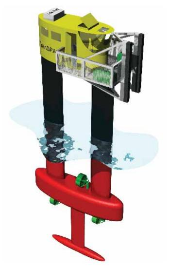
30% over vessels that are currently available. By enabling safe transfers at 3 meters, the propelled spar vessel is expected to increase access time to 310 days per year from 200 days per year currently.
