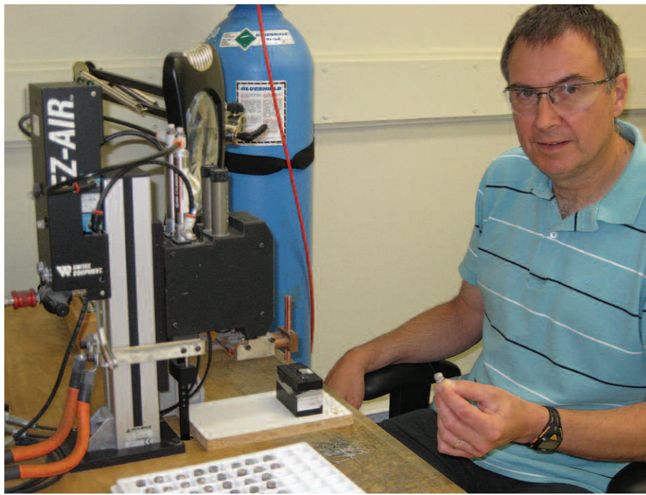
Lotek's general manager, Mark Ploughman, at the battery pack station where the company produces its own silver oxide battery packs. Photo: Andrew Safer
